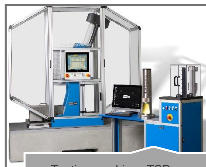
Testing machines TCR – comprehensive solution for impact testing
