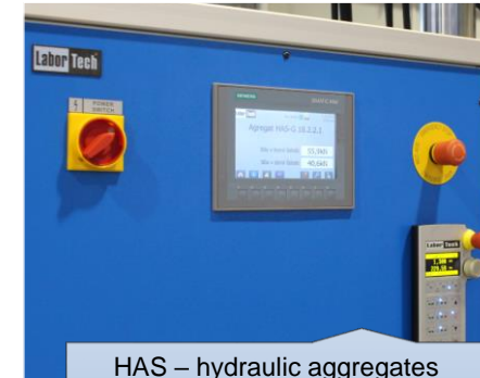
HAS – hydraulic aggregates designed for static tests with integrated diagnostics HALT 16 – Simatic.
