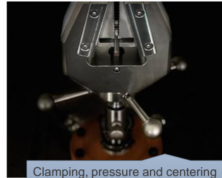
Clamping, pressure and centering fixtures. Selection according to nominal force, surface, test frequency, standard, etc.
