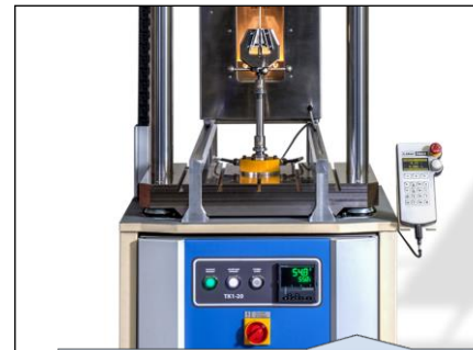
Temperature chambers with a range from - 196 ° C to + 350 ° C integrated in the EP series 1 machine
