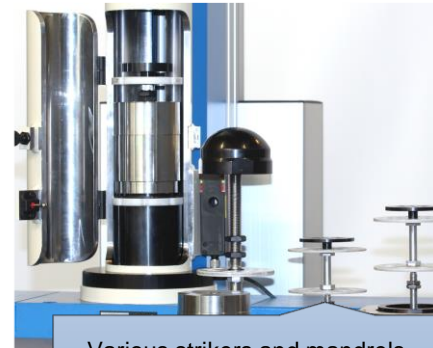
Various strikers and mandrels according to DIN, EN, ISO and ASTM norms and standards.
