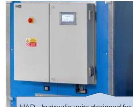
HAD - hydraulic units designed for dynamic tests with integrated diagnostics HALT 18 - Simatic.
