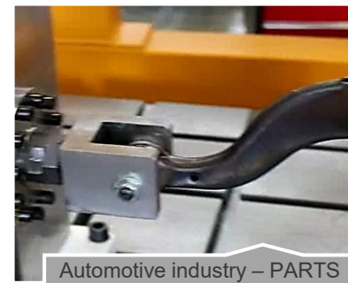
Automotive industry – PARTS multi-axis stresses on the body, components, shock absorbers, etc. under extreme conditions
