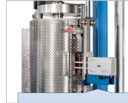
High temperature furnaces up to 1600 ° C.
