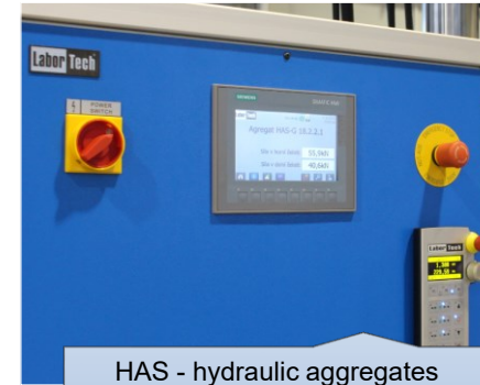
HAS - hydraulic aggregates designed for static tests with integrated diagnostics HALT 18 - Simatic
