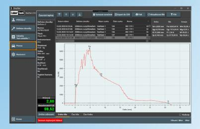
DROPTest Software for vertical impact tests – drop weight testers
